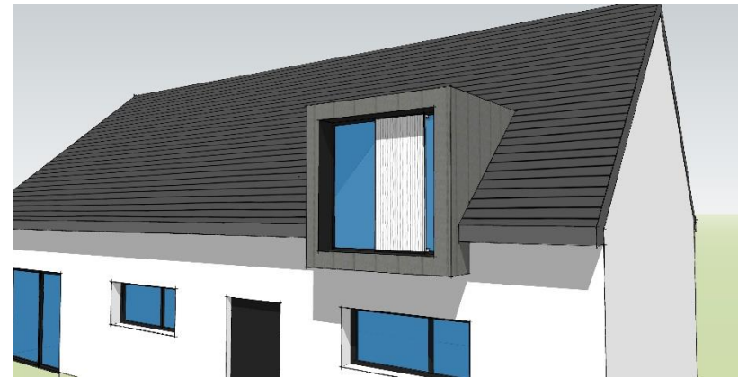
Figure 5.9 – Contemporary dormer in rear elevation
