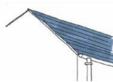
Figure 5.2 – Appropriate minimal roof edge treatment
