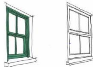
Figure 5.11 – Timber window and uPVC window.
