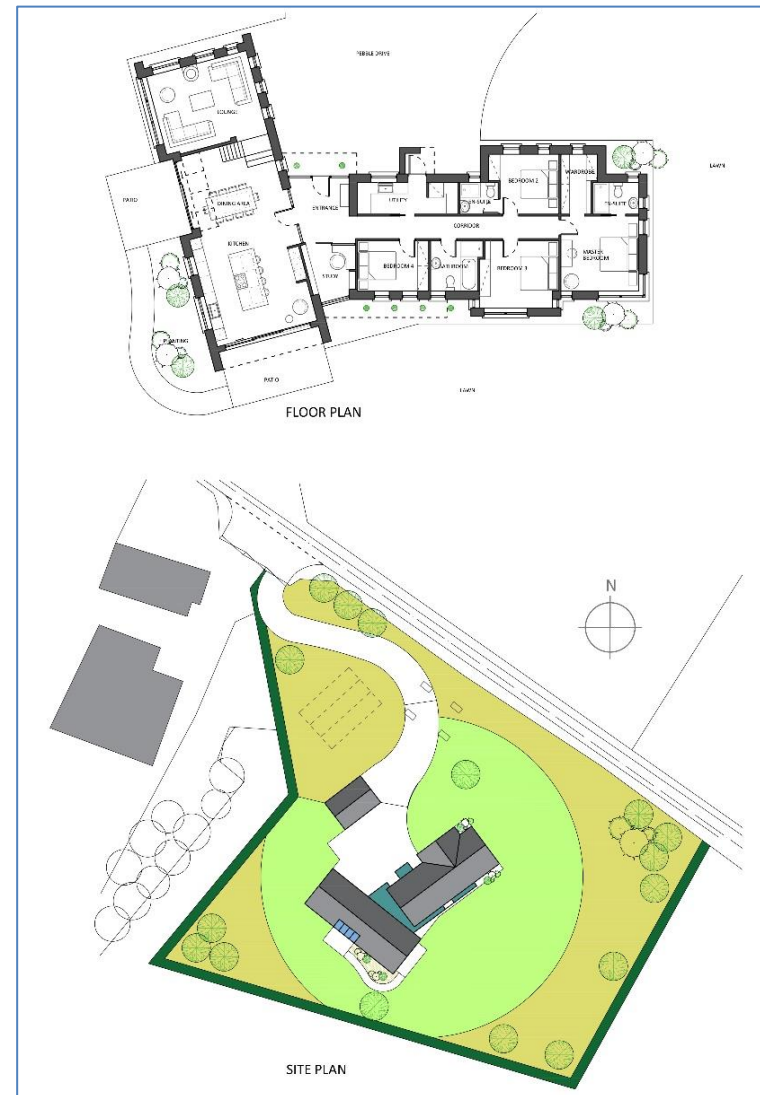
Figure 4.7 – Example of a floor plan and site layout for a single storey design proposal which breaks down the mass using narrow plan elements.
