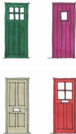
Figure 5.12 – Appropriate simple design vertical sheeted doors.
