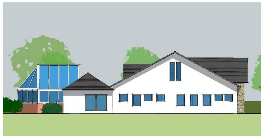
Figure 4.4 – Side elevation illustrating deep plan with all elements out of proportion to each other.
