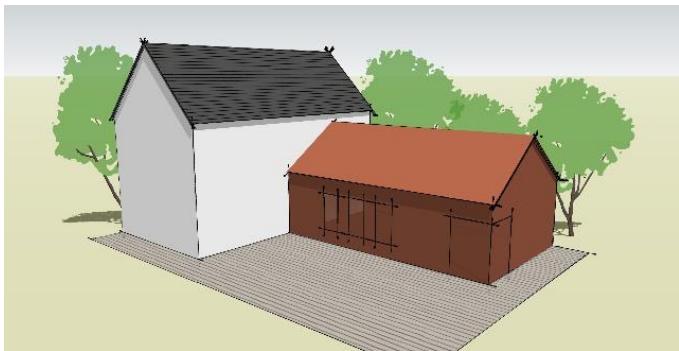
Figure 8.13 – 'L' shaped pitched roof extension
