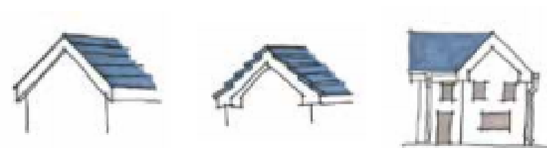
Figure 5.3 – Avoid roofs with large overhangs which result in the roof sitting like a 'lid' on the building.
