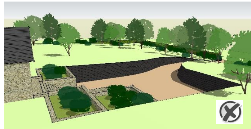
Figure 3.5: Example of excessive cutting to facilitate driveway.
