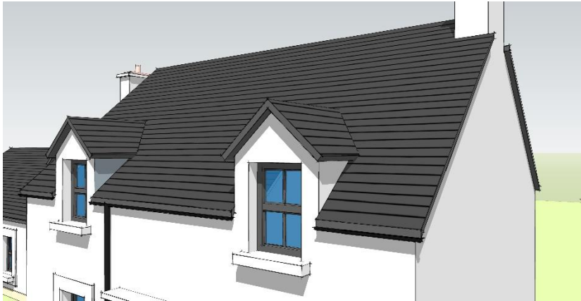
Figure 5.6 – Example of a well-designed dormer window projecting from the main wall
