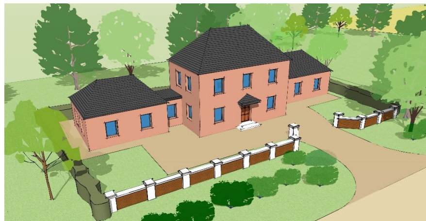
Figure 4.2 – An over-scaled dwelling in relation to plot and distance from site boundaries.
