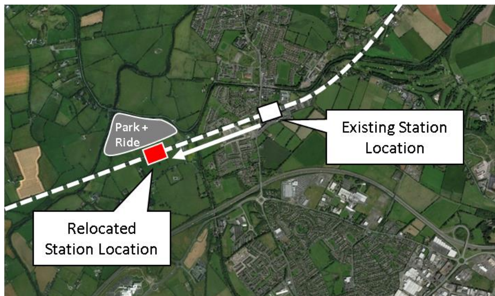
Figure 8.33 Rail Option 1: Relocating Station to the West
