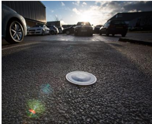
Figure 9.31 Example of a Parking Bay Sensor
