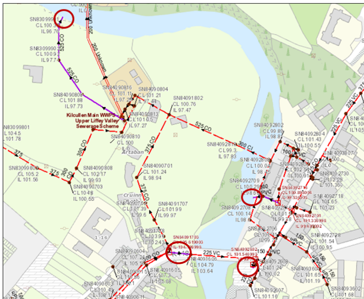
Figure 5-5 Foul Sewerage overflow to River Liffey (Circled in red) and surface & foul sewers interactions.
