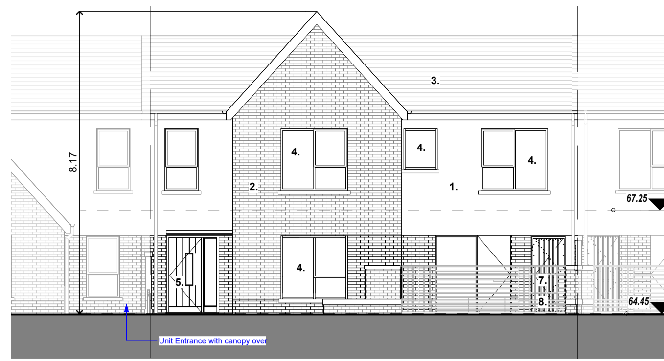
1 FRONT ELEVATION - UNIT TYPE D2 1 : 100
