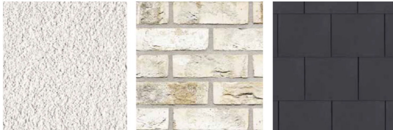
Image 14: Proposed primary materials of light coloured render (left), light coloured clay brick with off-white mortar (middle), and artificial roof slate/ roof tile (right). Refer to elevation drawings for details of other materials.
