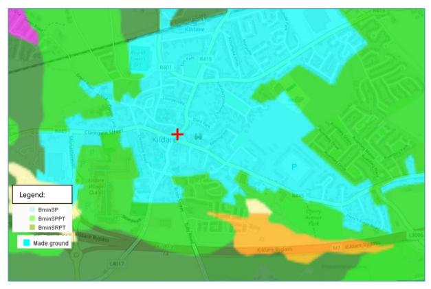
Figure 4: Subsoils in the context of the Subject site (Source: EPA Mapping)
