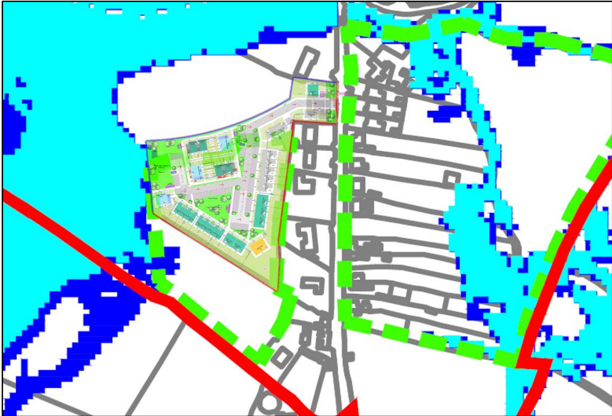
Figure 2-9: Approximate Overlay of Site Layout on Local Area Flood Risk Assessment Map
