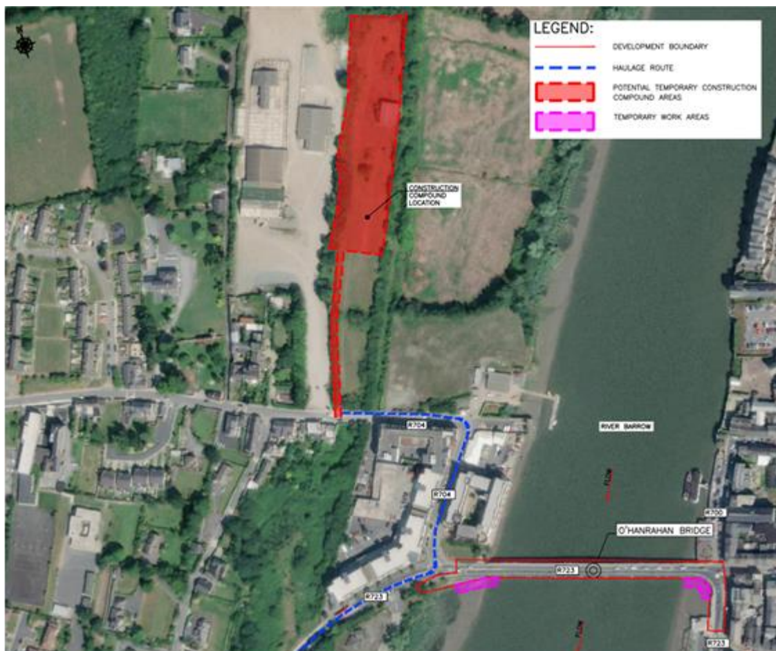
Plate 2-6 Location of the Construction Compound
