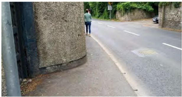
Figure 1-4: Clane Rd & English Row - Substandard Cross Section (Google Maps)
