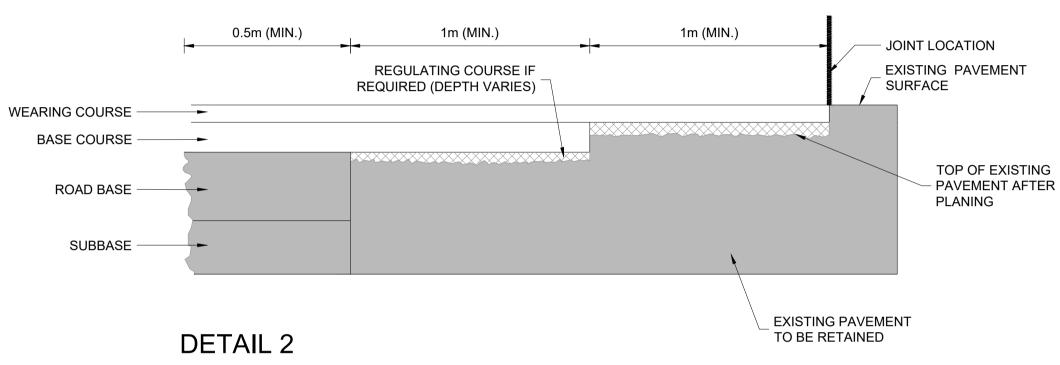
TYPICAL PAVEMENT JOINT DETAIL BETWEEN NEW CONSTRUCTION AND EXISTING ROAD (NOT TO SCALE)
