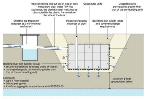
Figure 13.1 Soakaway details (including a pre-treatment system)
