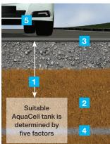
The combination of these 5 factors effectively means that the required characteristics of a geocellular structure to be installed under a trafficked location (for example) will be very different from that under a landscaped/low-loaded location.
