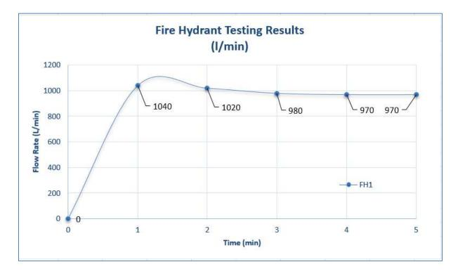
**Figure 3: Fire Hydrant Flow Test Results**
