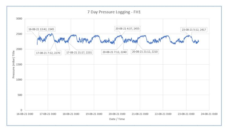
Figure 2: 7-Day Static Pressure Logging Results
