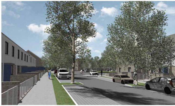
Above: View along central street, looking west. Carriageway and parking zones are clearly defined, with landscape strip between parking and pavement. Front curtilages are defined by a combination of steel gates and railings, and bin stores
