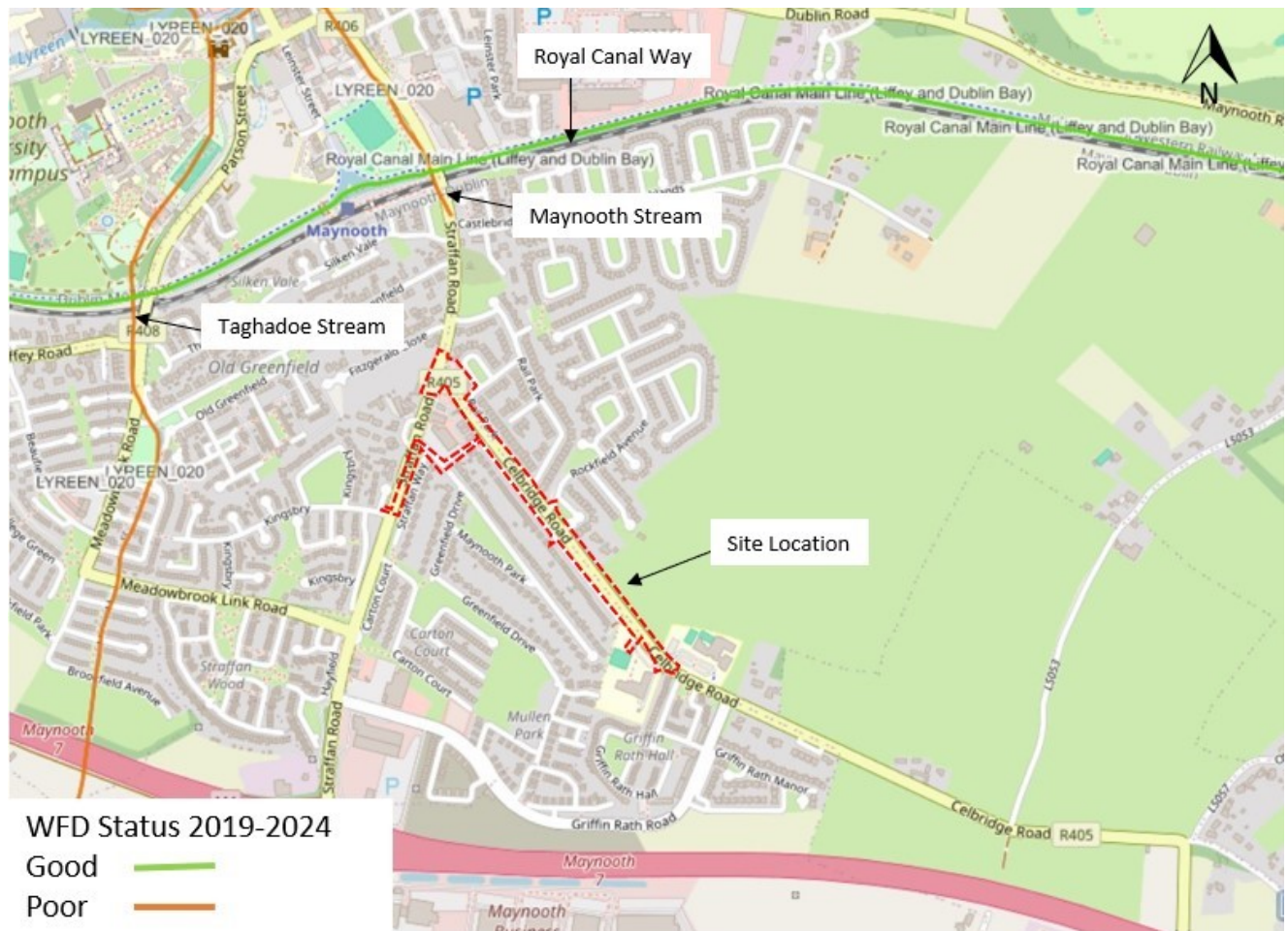
Figure 2-4 WFD Status of River Waterbodies within 500 m of site location (EPA, 2026)
