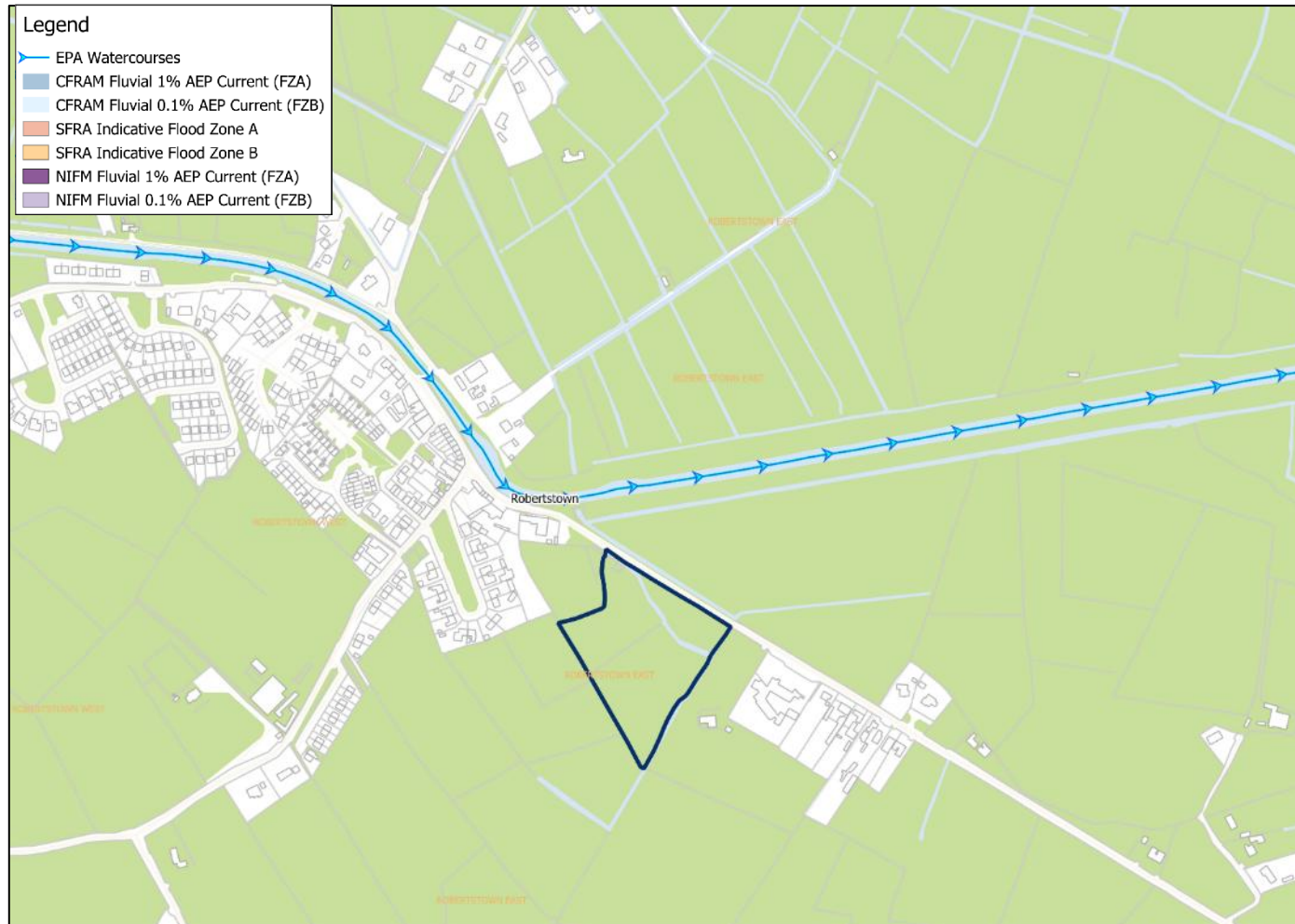
Figure 12: MA No. 23 Robertstown Land Use Zoning Map Amendments overlain with Flood Zone Sources
