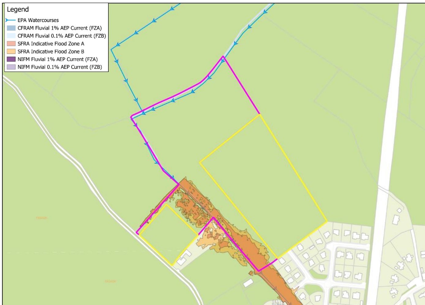
Figure 10: MA No. 21 Kildangan Land Use Zoning Map Amendments overlain with Flood Zone Sources
