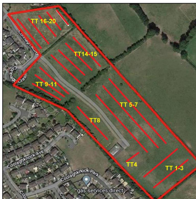
Figure 5: Test trench layout
