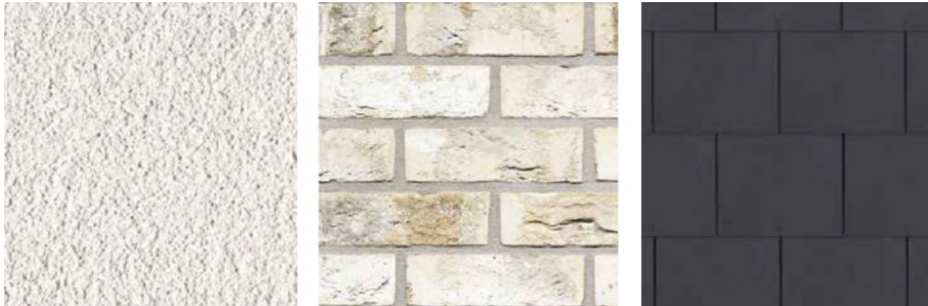
Image 23: Proposed primary materials of light coloured render (left), light coloured clay brick with off-white mortar (middle), and artificial roof slate/ roof tile (right). Refer to elevation drawings for details of other materials.
