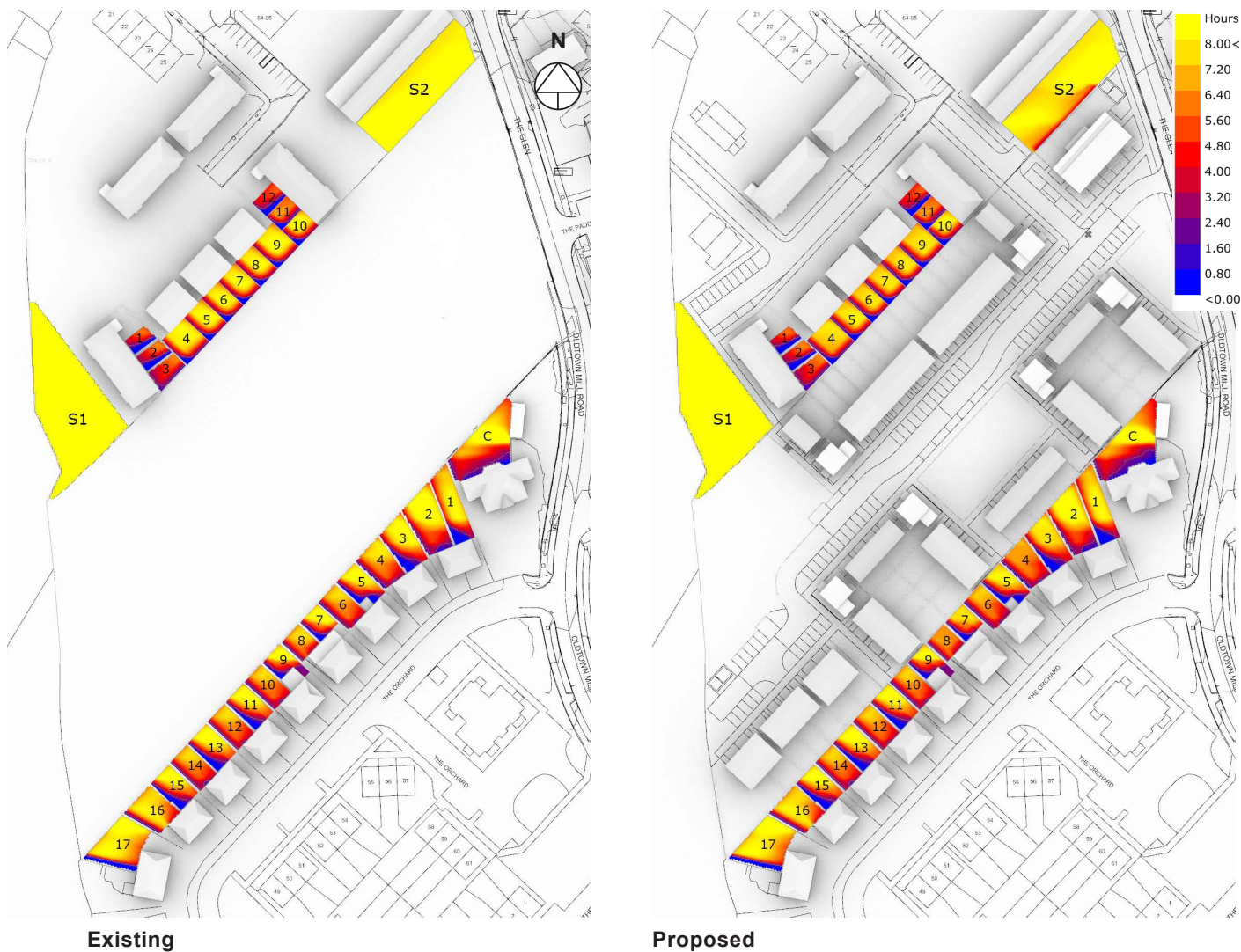
Figure 5: Existing & Proposed Radiation map of amenity areas, showing available sunlight on 21st March. The scale represents the percentage of daylight received from 0 - 8 hrs.
