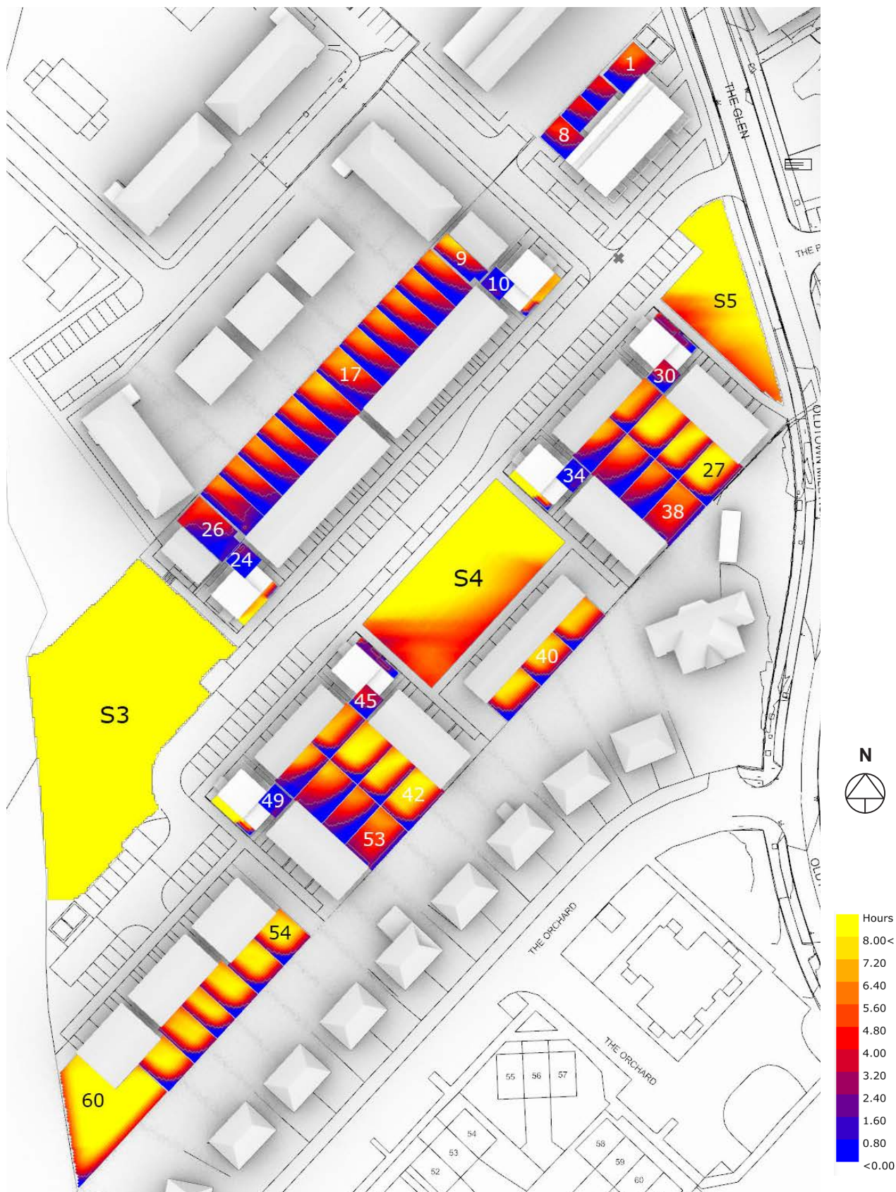
Figure 6: Radiation map of amenity within the Proposed Development, showing available sunlight on 21st March. The scale represents the percentage of daylight received from 0 - 8 hrs.
