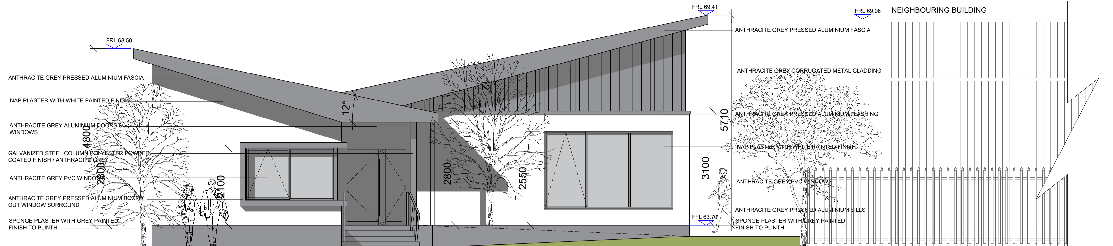
NORTH WEST ELEVATION
