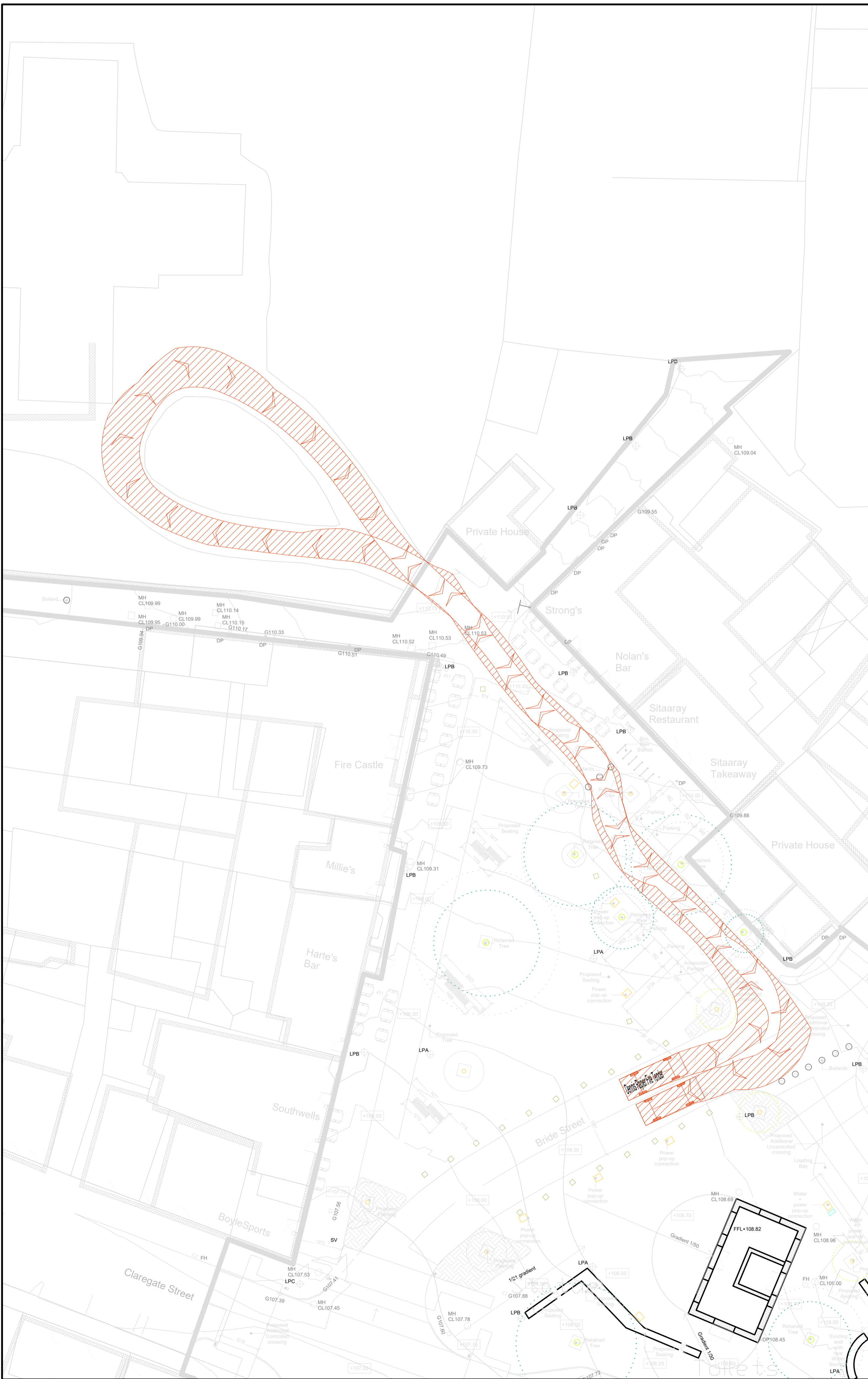
A PROPOSED SWEEP PATH ANALYSIS WITH FIRE TENDER 0005 Scale: 1:250
