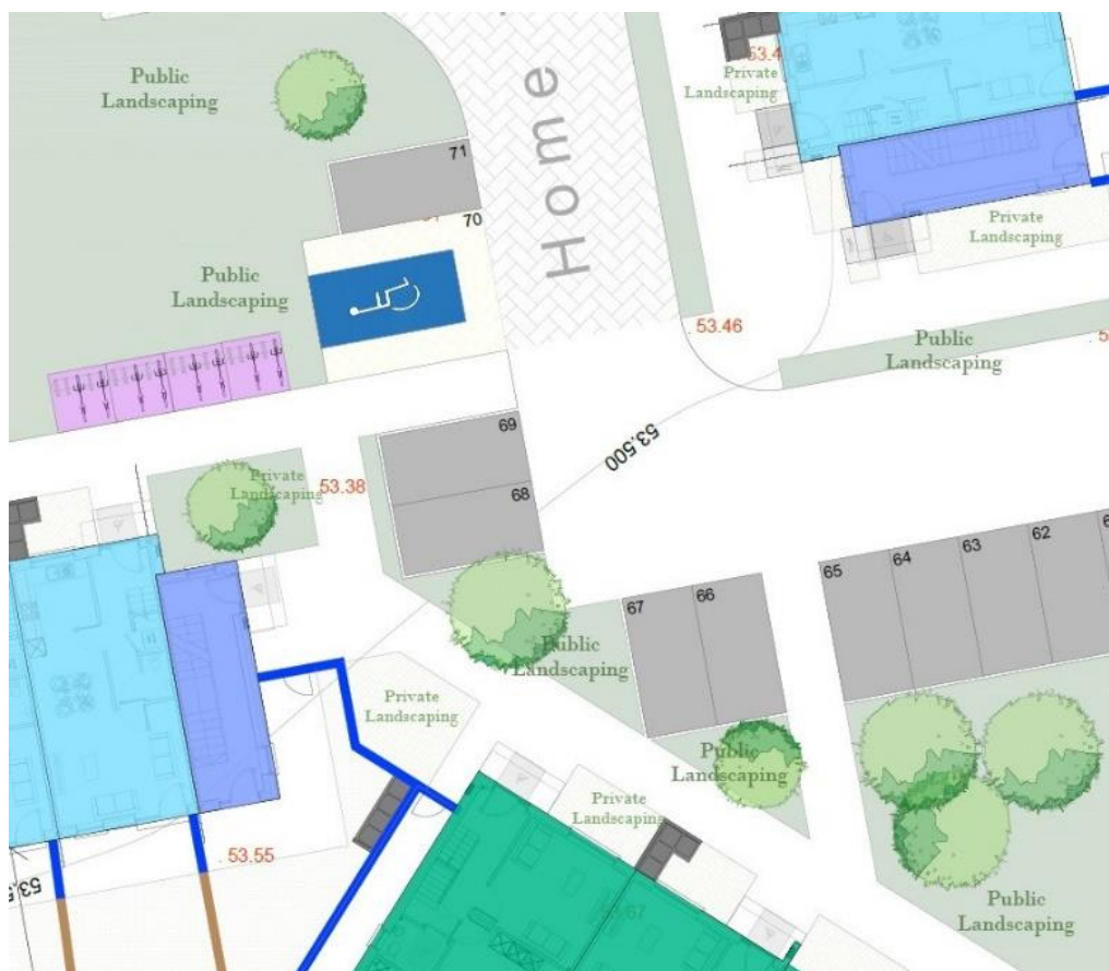
Fragment of the Site Plan, showing Landscape including public landscaping and private landscaping, to buffer the approach to individual units
