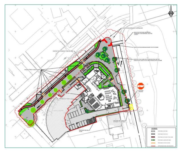
Figure 2: Proposed General Arrangement (Source: AECOM Drawing 606669624-ACM-XX-00-DR-CE-10-0001)
