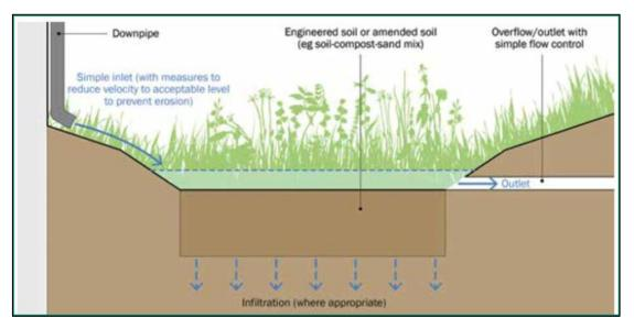
Figure 10: Typical Bio-Retention Section (Source: CIRIA C753 SuDS Manual)
