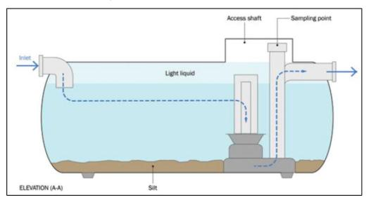
Figure 12: Typical Petrol Interceptor Detail (Source: CIRIA C753 SuDS Manual)
