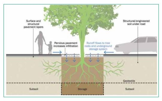
Figure 11: Collection of Surface Water Runoff for Trees (Source: CIRIA C753 SuDS Manual)
