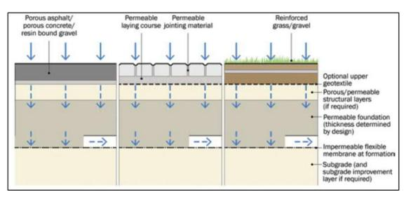
Figure 9: Porous Surfacing System - No Infiltration (Source: CIRIA C753 SuDS Manual)
