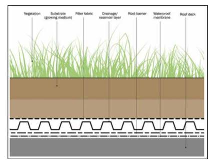
Figure 8: Typical Section through Extensive Green Roof (Source: CIRIA C753 SuDS Manual)
