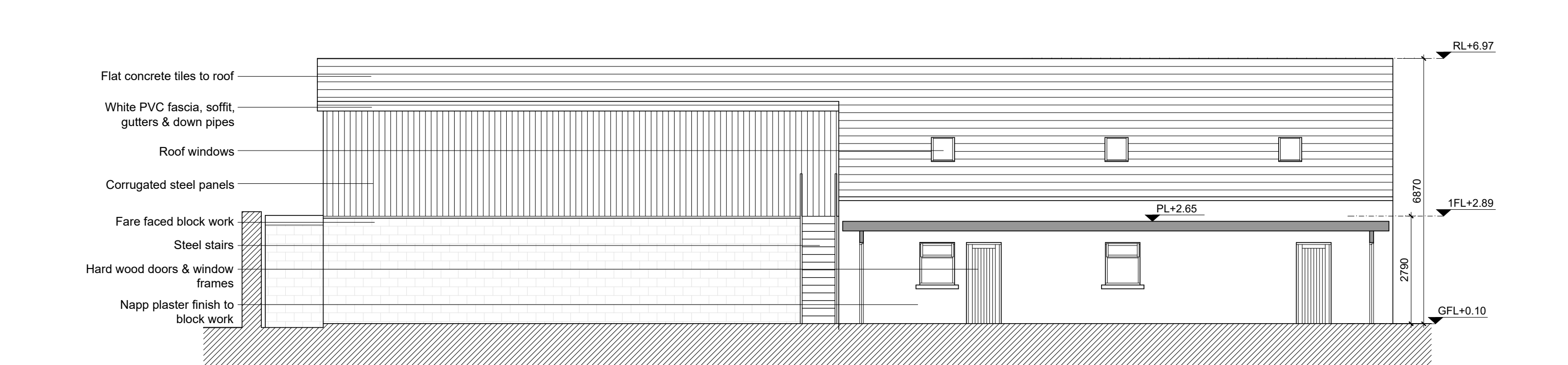
4 EXISTING NORTH FACING ELEVATION SCALE 1:100
