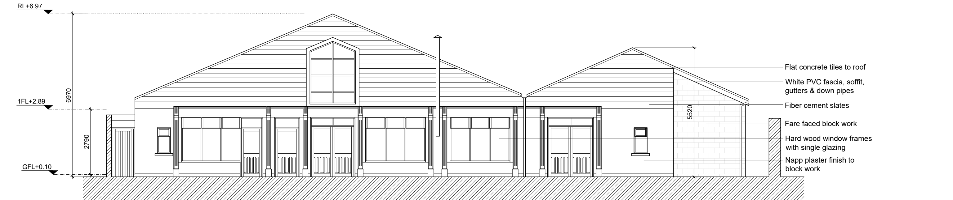
2 EXISTING WEST FACING ELEVATION SCALE 1:100
