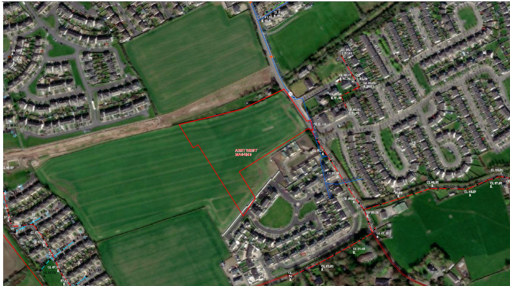
Figure 3.6 Existing Watermain, Foul & Surface Water Network
