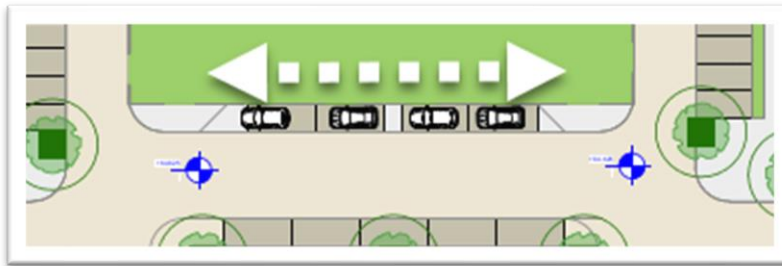
Figure 2.5 – Footpath Terminating Each Side of Parking
