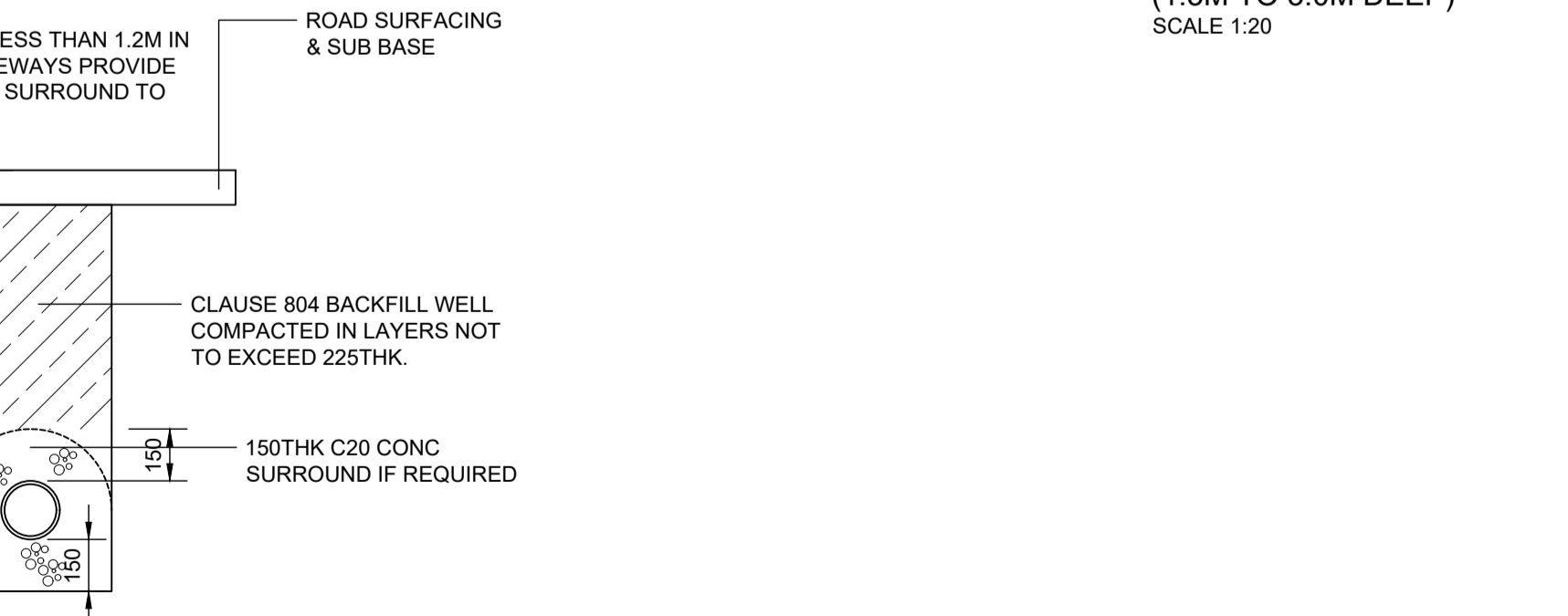
TRENCH BEDDING (FLEXIBLE PIPEWORK IN ROADWAYS) SCALE 1:20
