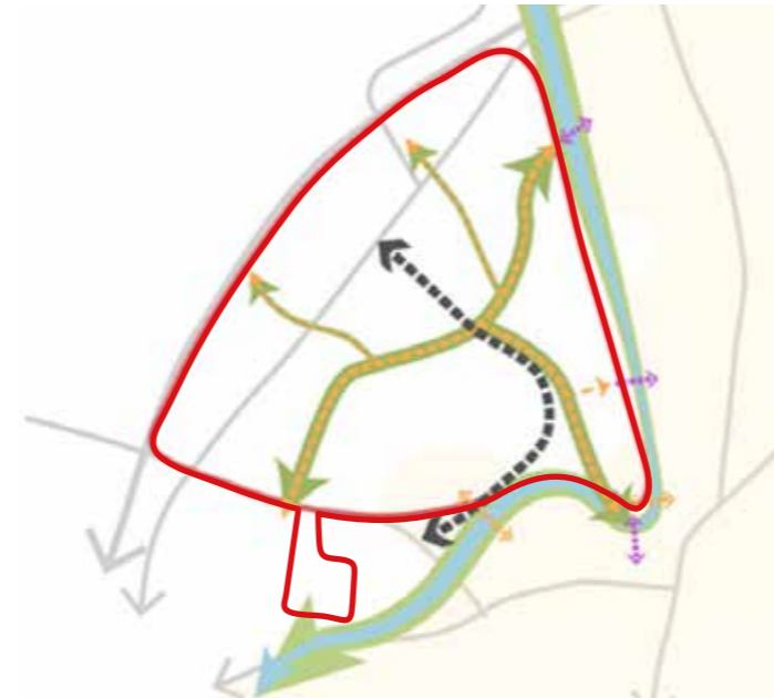
Option B - Link Millennium Park Road to New Caragh Road using the existing Old Caragh Road alignment.
