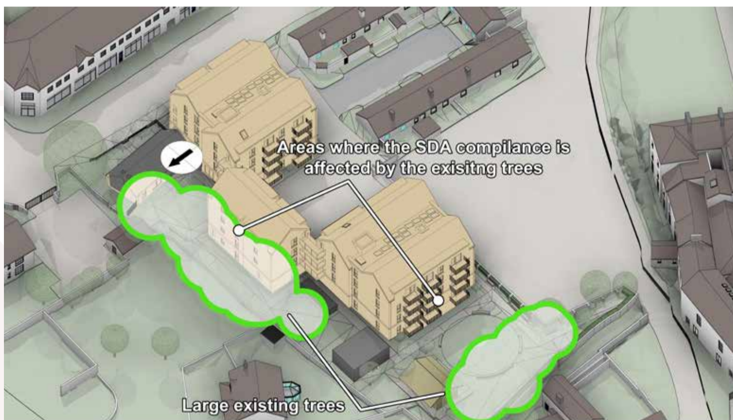
Figure 3.3: Areas within the blocks where SDA compliance is affected by existing trees.
